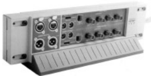
A typical breakout box (this, from Media 100 circa 1995), with balanced audio in/out on the left, component video in/out on the right, and composite in/out nestled between.
