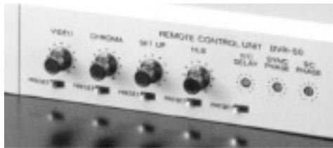
Timebase corrector controls (left) provide an editor with knobs for adjusting hue, chroma, etc.; the output from the video deck (right), however, offers component, composite and S-video—each within its own color space.
